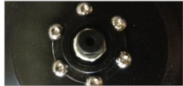
Disc bolts go on the left of the bike
